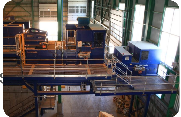
X-Ray and NIR optical sorter to clean the organic
